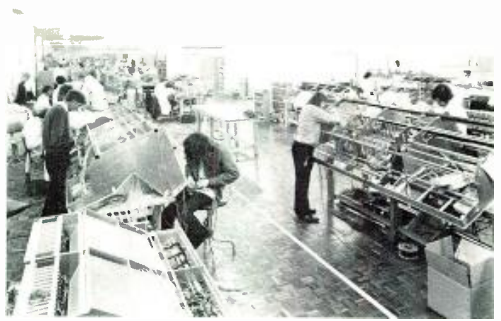
Wiring shop. Approximately fifty consoles are under construction at any one time in the Neve factory.
