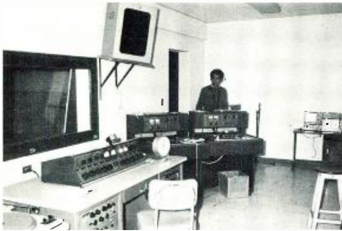
In this view of control room 2, we can see the Altec console and speakers, Pultec equalizers, and two Ampex 354 recorders in custom made cabinets. At the rear can be seen the movable test equipment rack (on a typewriter table) consisting of a group of Sennheiser and Grundig components.
